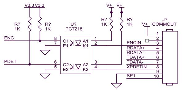
Each input requires the capability of sinking 12ma to ground as depicted in the above circuit. Connection to the optional control port requires an RJ50 connector.
