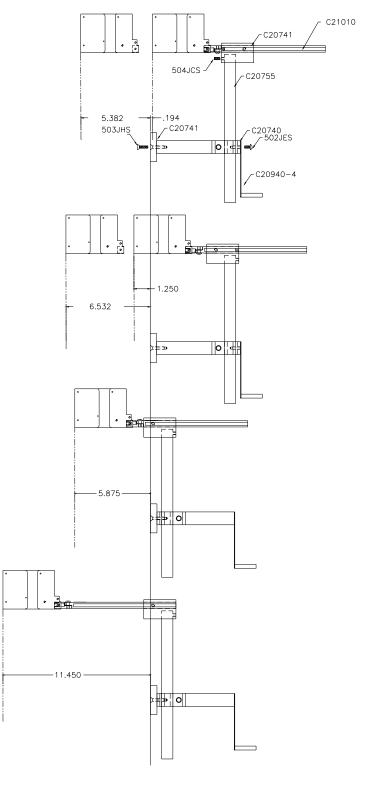
Vertical height adjustment for the EVOLUTION II print head is accomplished by loosening the included hand knob 5993K41.
