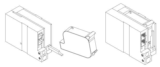
NOTE: WHEN A NEW CARTRIDGE IS INSTALLED, BOTH THE RED AND GREEN LIGHT WILL FLASH TWICE INDICATING A CORRECT INSTALLATION. THE USER MUST REMEMBER TO RESET THE INK LEVEL UNDER THE F4 FUNCTION KEY.
