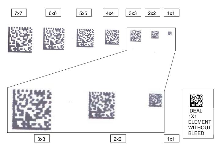
As a comparison the following is a scanned image of the actual printed sample.
