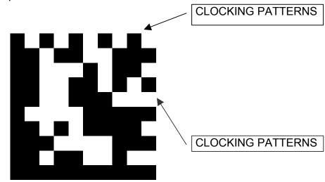
Data matrix codes are more tolerable to stretch and skew by the nature of their imbedded clocking patterns defining both columns and rows.
