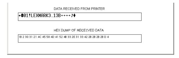
The bottom half of the display shows the ASCII data received from the printer and the hex values for the received data displayed in the last text box.
