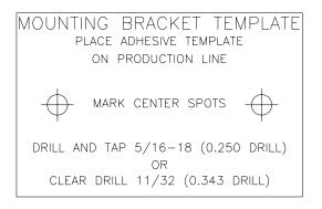
Locate the supplied mounting template and affix in a convenient location on the production line. Spot and drill both mounting holes for a 5/16" bolt. NOTE: the user may also thread the side of the conveyor using a 5/16" tap.
