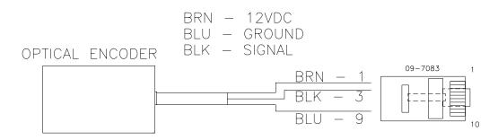
The above pictorial is an example of the connections for an external encoder.
