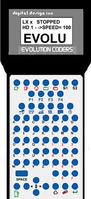
The keypad on the print station, pictured here, contains 64 keys. The LCD will display various messages to assist in programming on the upper half of the display. The lower half of the display will show the actual message in a WYSIWYG (What You See Is What You Get) format.
