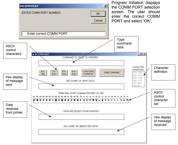
After a comm. Port is selected the above screen is displayed. This program allows for simple command entry and provides the programmer a detailed view of both the characters sent and the data received from the printer.
