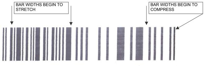
Finally, the image as it should look. This code was produced on white corrugated at 100ft/min and produced a verifiable class "A" barcode with a decodability of 70%. The average bar growth from the reference standard was 0.03%.
