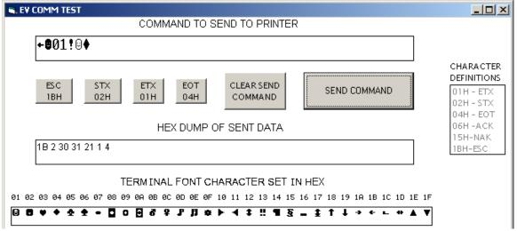
When the "SEND COMMAND" button is selected the second text line displays the hex values of the message sent to the printer. In this case the ASCII character ! (Exclamation Point) was sent to the printer. This command requests the printer to respond with the software version of the system.
