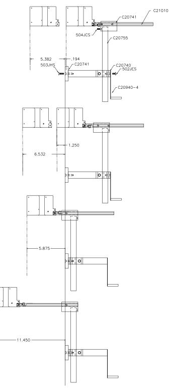
Vertical height adjustment for the EVOLUTION LX print head is accomplished by loosening the included hand knob 5993K41.
