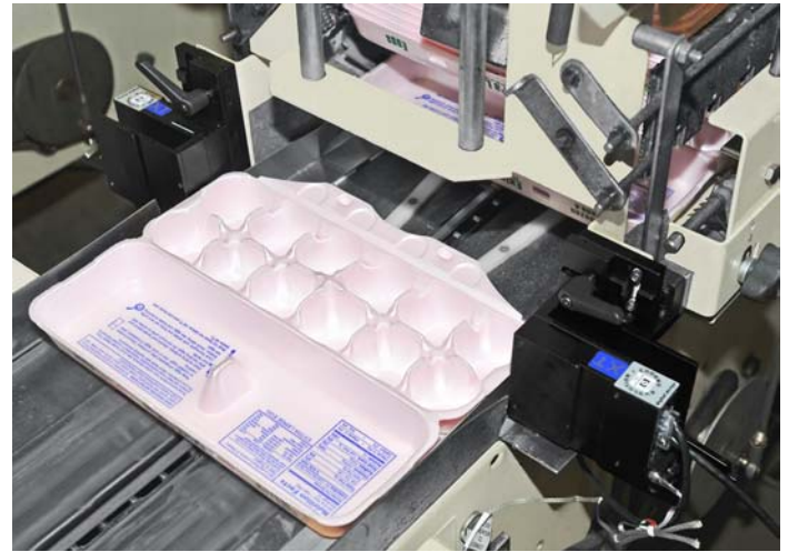
Evolution DM with 2 printheads shown mounted on an 8200 Diamond Machines egg packager.
